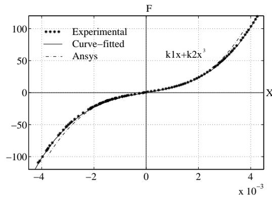
Figura 5: Relationship between loading and deformation
