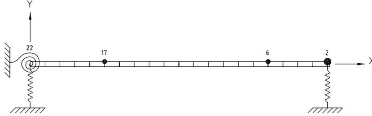
Figura 3: Analytical linear model Test Rig
