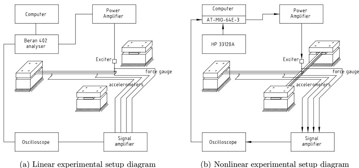
Figure 2: Block diagrams of the experimental setup Test Rig
