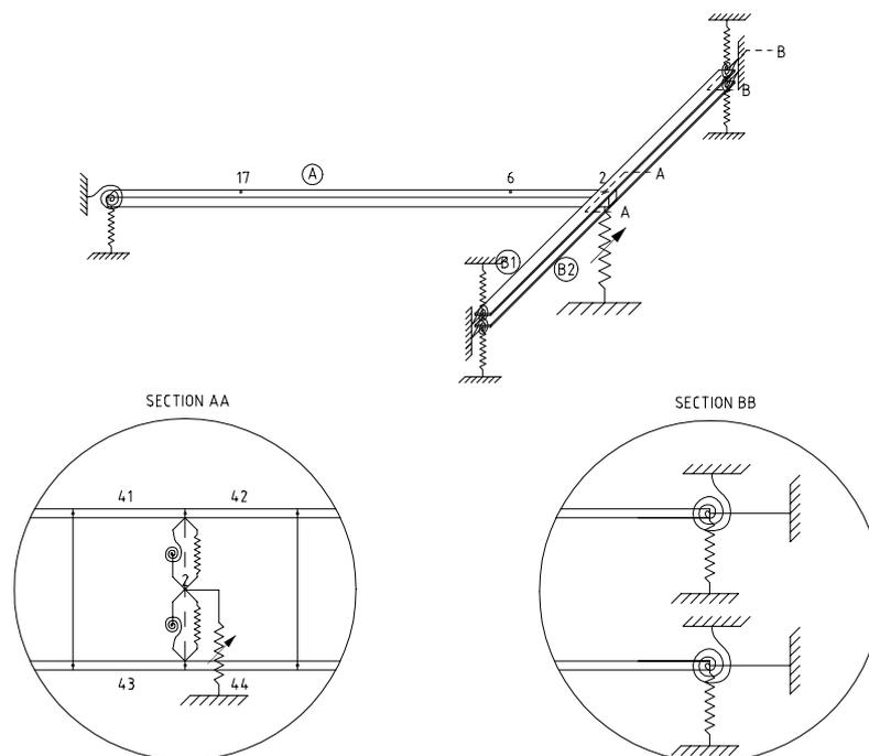
Figura 6: Analytical model Test Rig
