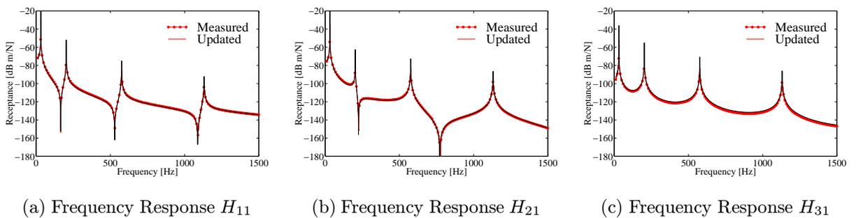
Figura 4: Frequency Responses of linear structure
